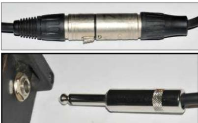
The 1/4” male plug (right) and 1/4” female jack (left) are used in line level and speaker system integration.
