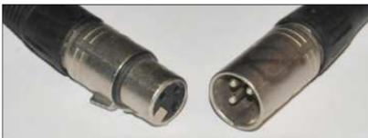
Microphone connectors exist as both female (left) and male (right). Two males or two females cannot join to create a connection. Only a male and female can (below).
